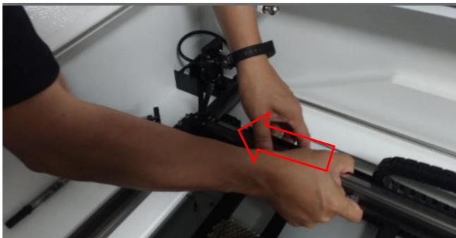
The last test is to touch these three wheels, the wheel should not be freely rotate by hand. If any wheel can be rotated, please re-assembly again.
